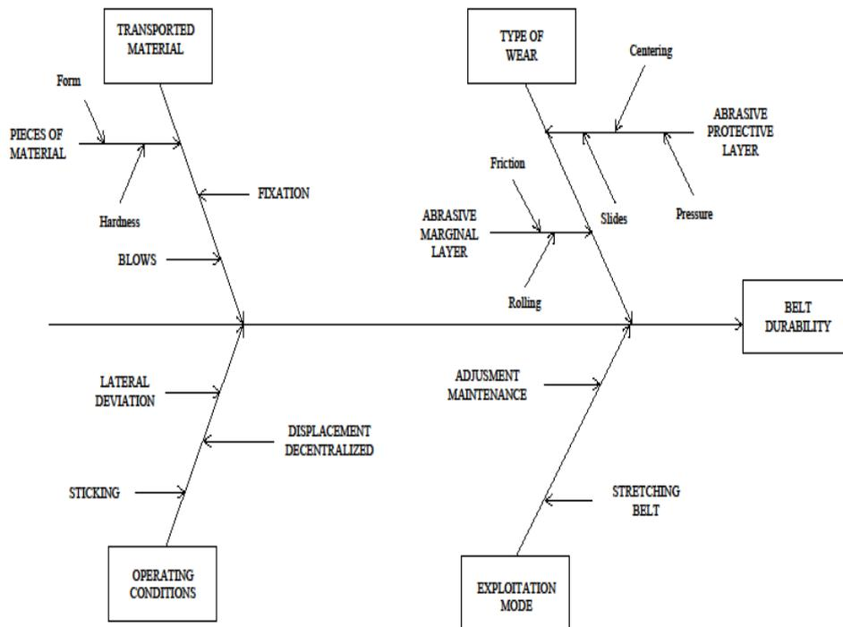
Fig. 3. Cause-effect diagram to identify belt durability
